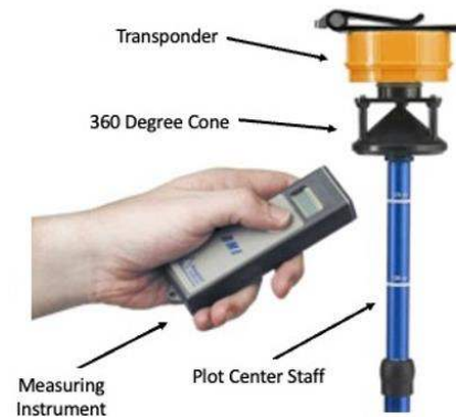
Figure 6.2.2a Distance Measuring Equipment (DME) 2
