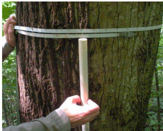
Figure 6.2.2b. Using a DBH tape and a pole to measure the tree diameter 3 .
